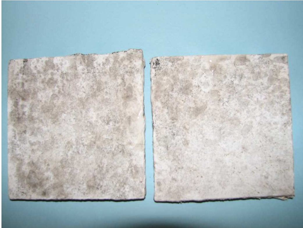
Plate 1: Fungal Resistance Test – PRA Control at 56 days
