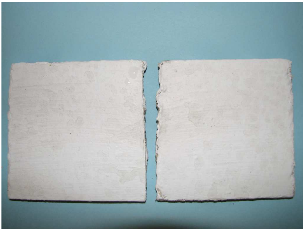
Plate 2: Fungal Resistance Test – Smaltoplast Silk at 56 days
