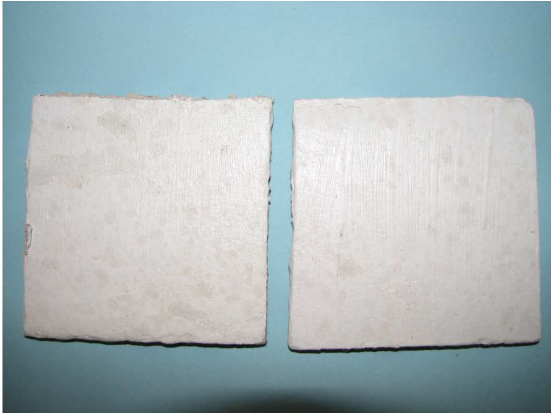
Plate 3: Fungal Resistance Test – Comparison Paint at 56 days
